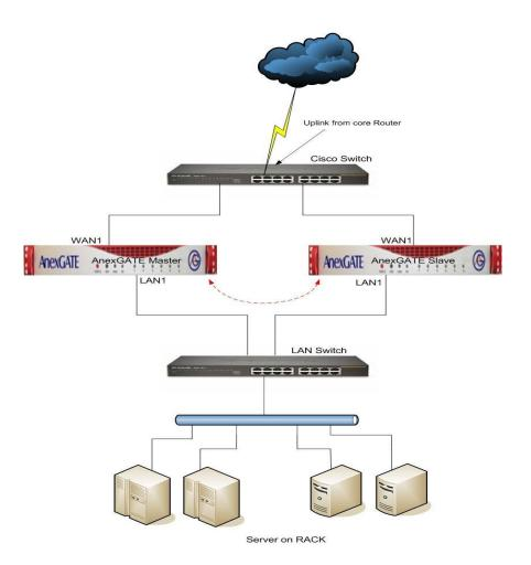
Note: The switches can be managed or unmanaged. Different switches for WAN and LAN is the only requirement.
